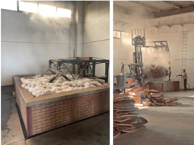
▲ The cork oak boiler bubbling away in the corner of the factory and cork being removed from the boiler. 2nd photo courtesy of our tour guide, Ana Veran.
