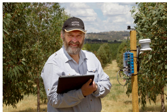
Cris with a tablet computer alongside an automated micro-climate station. Records from the station indicate trends expected in the tree measurements.
